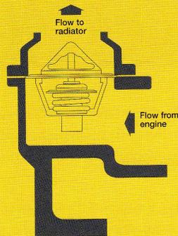
Figure 5 - Correct application for non Bypass Thermostat
