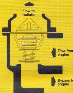
Figure 3 – Wrong Bypass Thermostat used engine runs hotter
