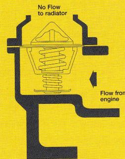
Figure 6 - Wrong application for Bypass Thermostat
