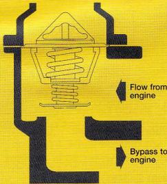
Figure 1 – Bypass Thermostat in correct position. On start up cold position restricts flow to radiator
