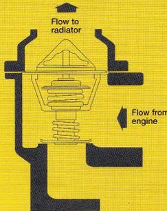
Figure 2 – Bypass Thermostat in correct position at normal operating temperature allows flow to radiator
